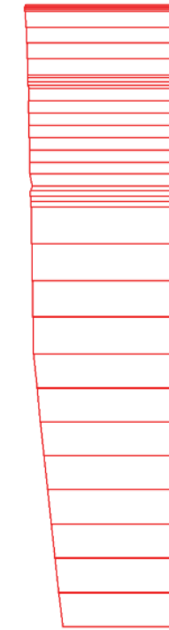
Fig. 28 Vertical displacements in beam (plate no: 6) Extreme value -52,55 \cdot 10^{-3} m (phase: 1)
