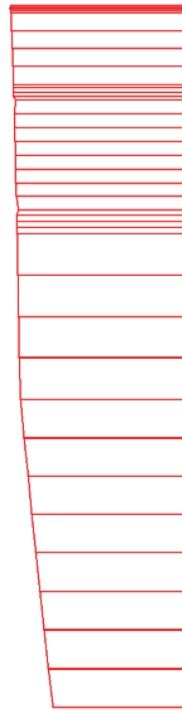
Fig. 29 Vertical displacements in beam (plate no: 5) Extreme value -52,53 \cdot 10^{-3} m (phase: 1)
