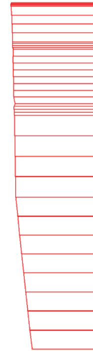
Fig. 28 Vertical displacements in beam (plate no: 6) Extreme value -52,55 \cdot 10^{-3} m (phase: 1)
