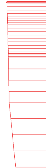
Fig. 28 Vertical displacements in beam (plate no: 2) Extreme value -52,38 \cdot 10^{-3} m (phase: 1)
