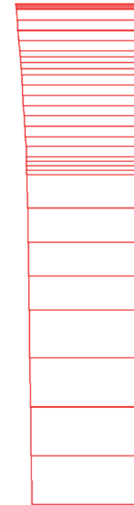
Fig. 128 Vertical displacements in beam (plate no: 2) Extreme value -334,87 \cdot 10^{-6} m (phase: 5)
