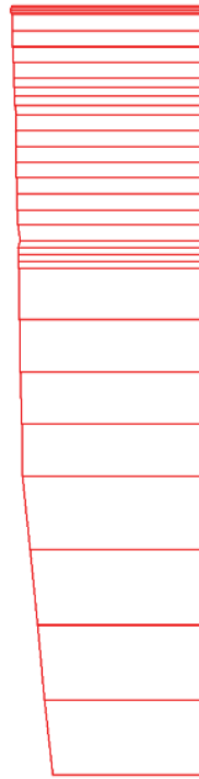
Fig. 29 Vertical displacements in beam (plate no: 1) Extreme value -52,37 \cdot 10^{-3} m (phase: 1)
